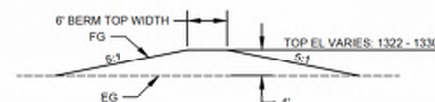
G BERM TYPICAL SECTION
